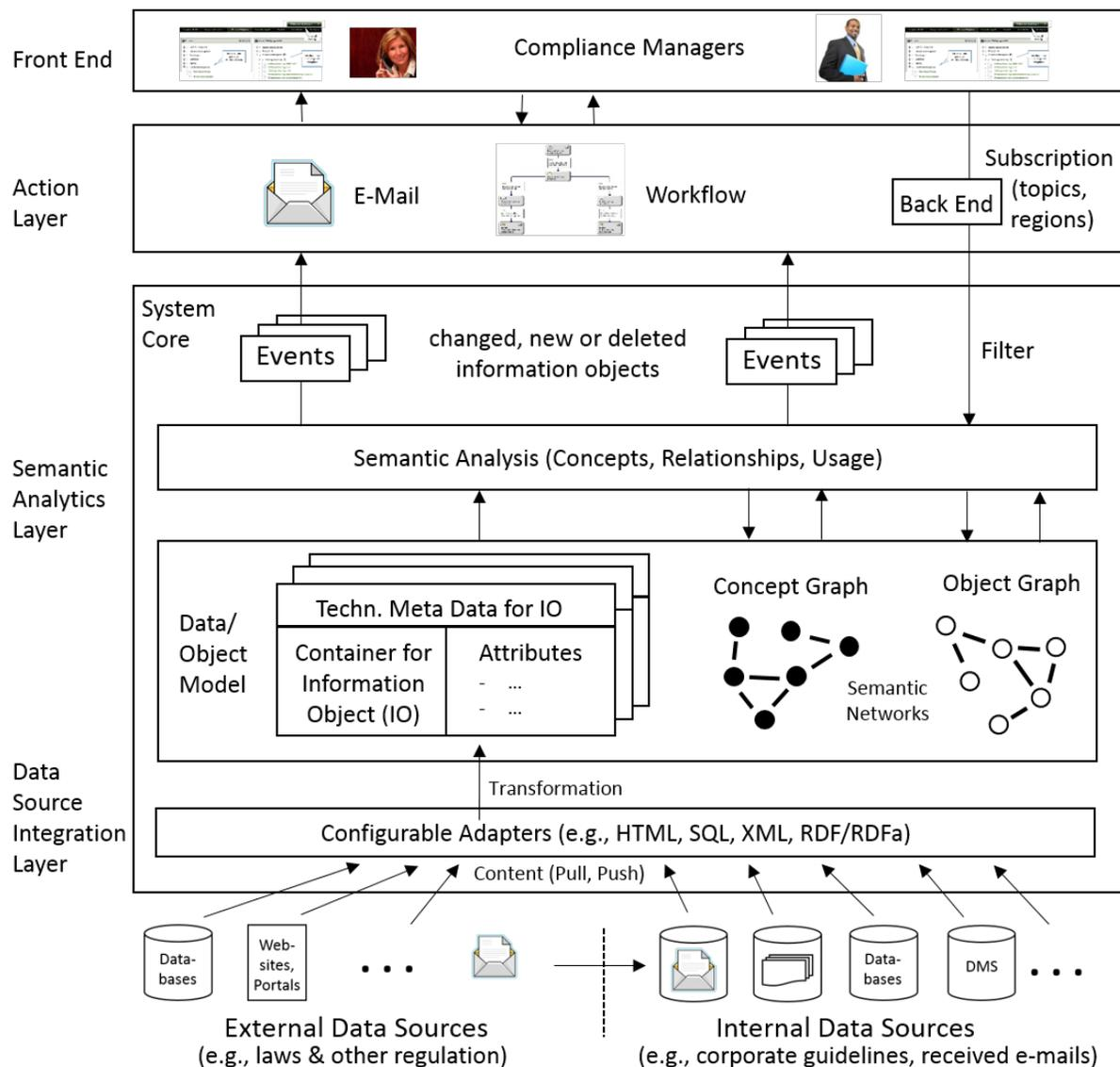
Fig. 1: Architecture of Compliance Activator
